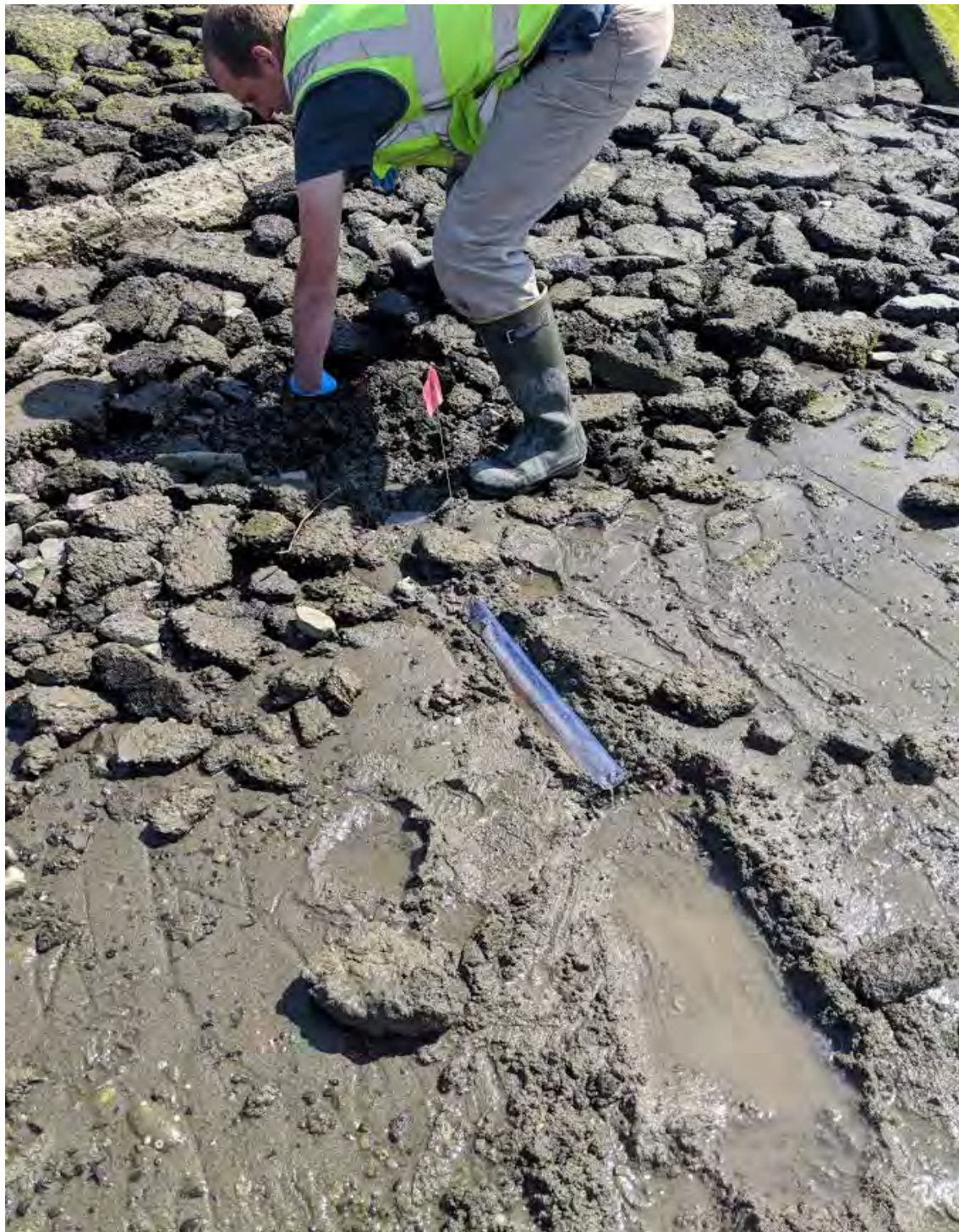
Example of Seep Sampling Set-up
