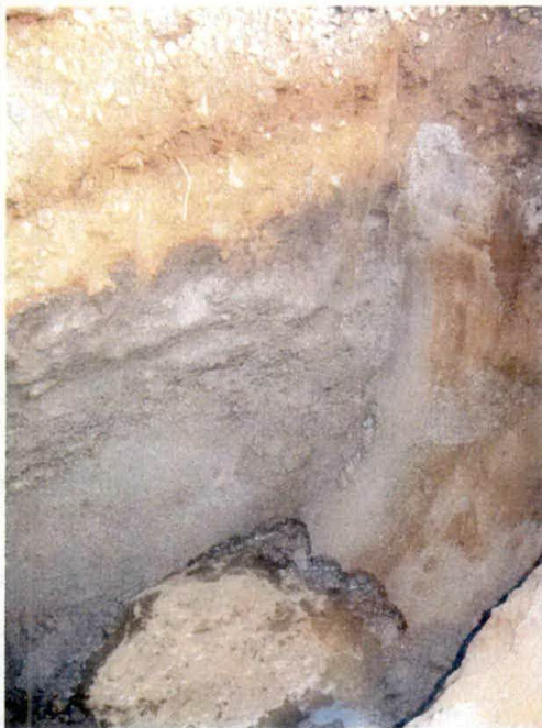
Photo 1: Grey sandy soil noted in TP4 displaying petroleum odors. Sample TP4 collected from this material.
