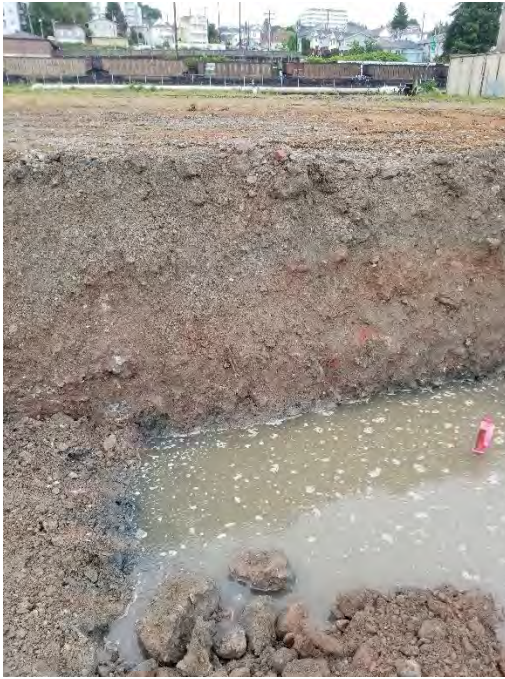
Photograph 1. Approximately 3 feet of CM overlying soil at the PM-B-6 Area, view looking east.
