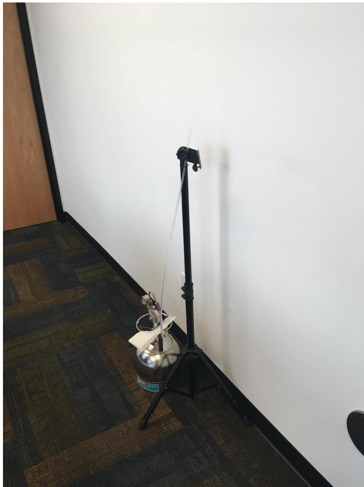
Photograph 4. Indoor air sample collection in Building A break room enclosure (sample IA-A1).
