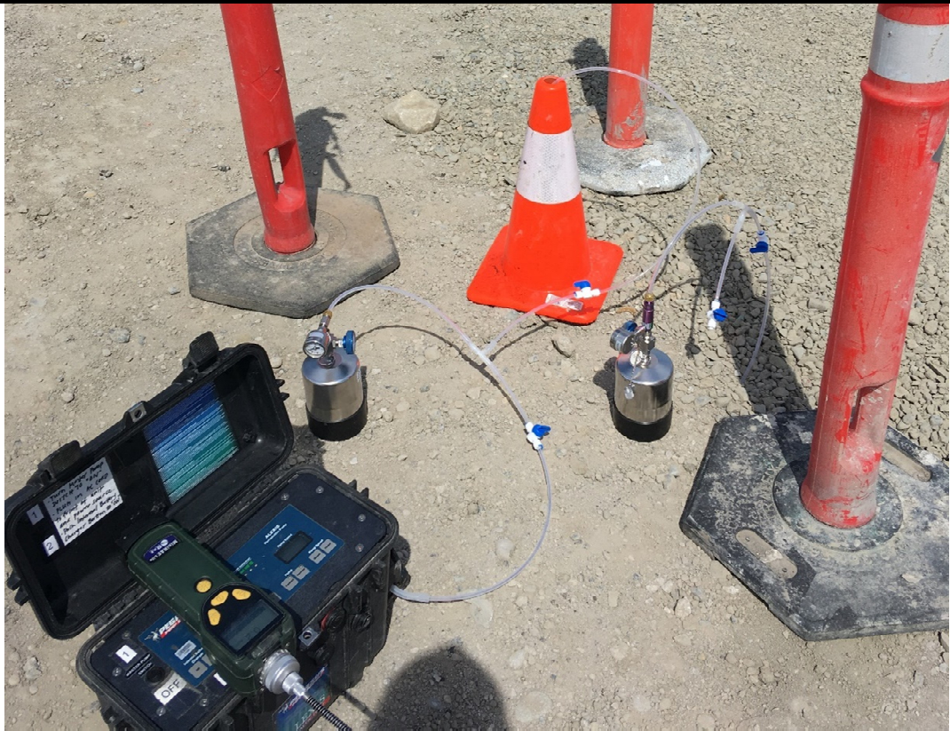
Photograph 9. VOC vapor sampling equipment.
