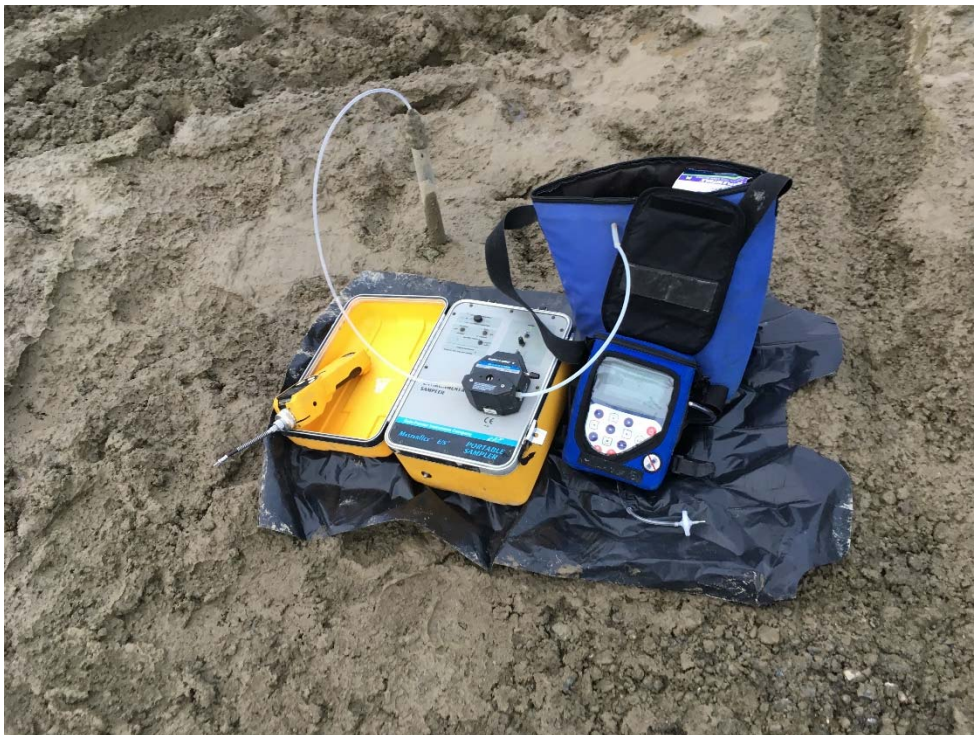
Caption: Purging post-run tubing sample point with peristaltic pump
