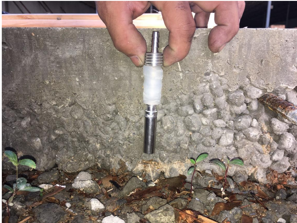
Photograph 1. Soil vapor pin with extension next to slab for comparison.
