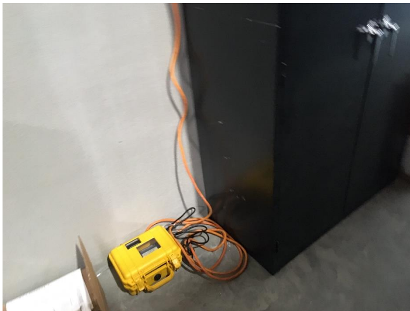
Photograph 2. Cross-slab differential pressure data logger with 0.001 inches of water resolution.
