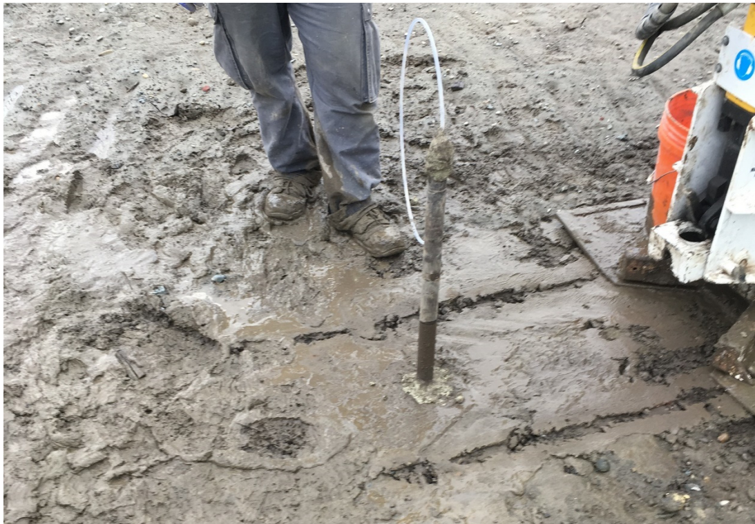
Photograph 8. Vapor sampling set up in May 2018.
