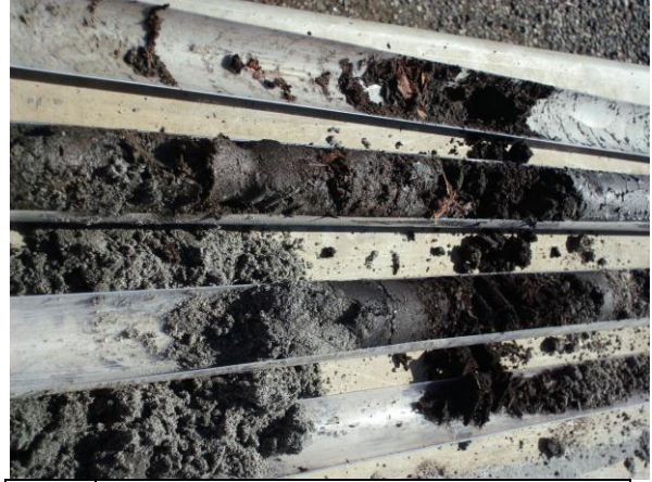
Photo #14: View of soil core samples collected from boring B-8. Upper cores denote soft wood debris materials from 8 to 10 feet bgs.
