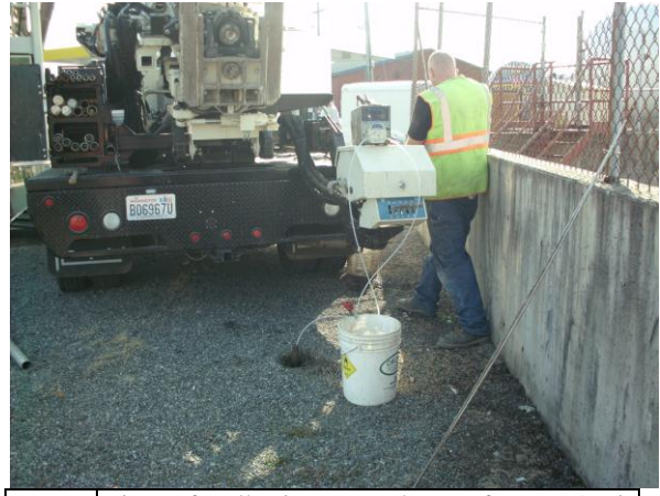
Photo #2: View of collecting groundwater from B-1 via peristaltic pump (looking east).
