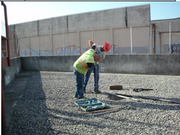
Photo #3: View of hand probe activities at boring B-2 (where the former 70k gal fuel tank was located) via a rotor hammer (looking west).
