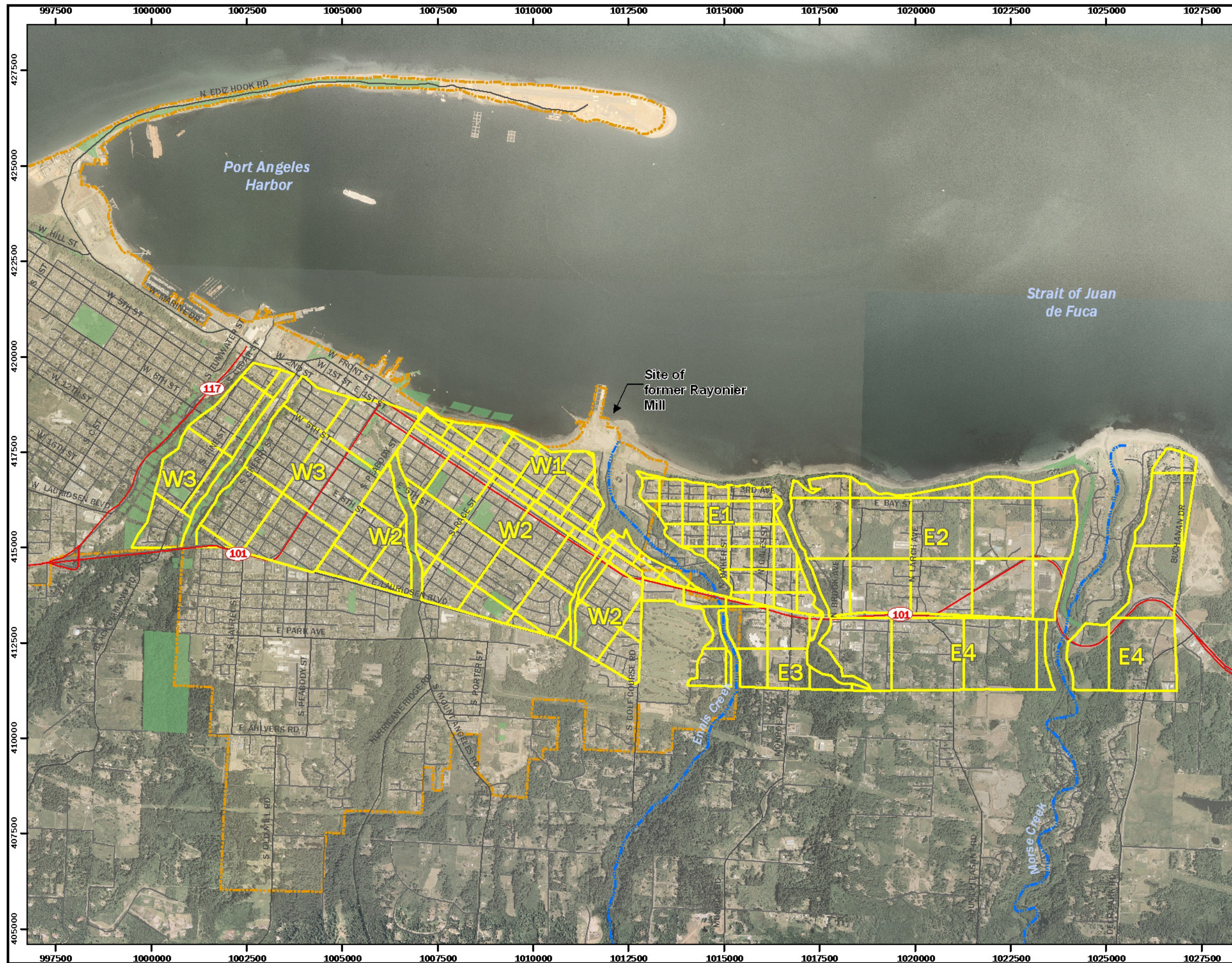
Figure 5-2 Sample Grid Spacing Rayonier Mill Off-Property Soil Dioxin Study Port Angeles, WA
