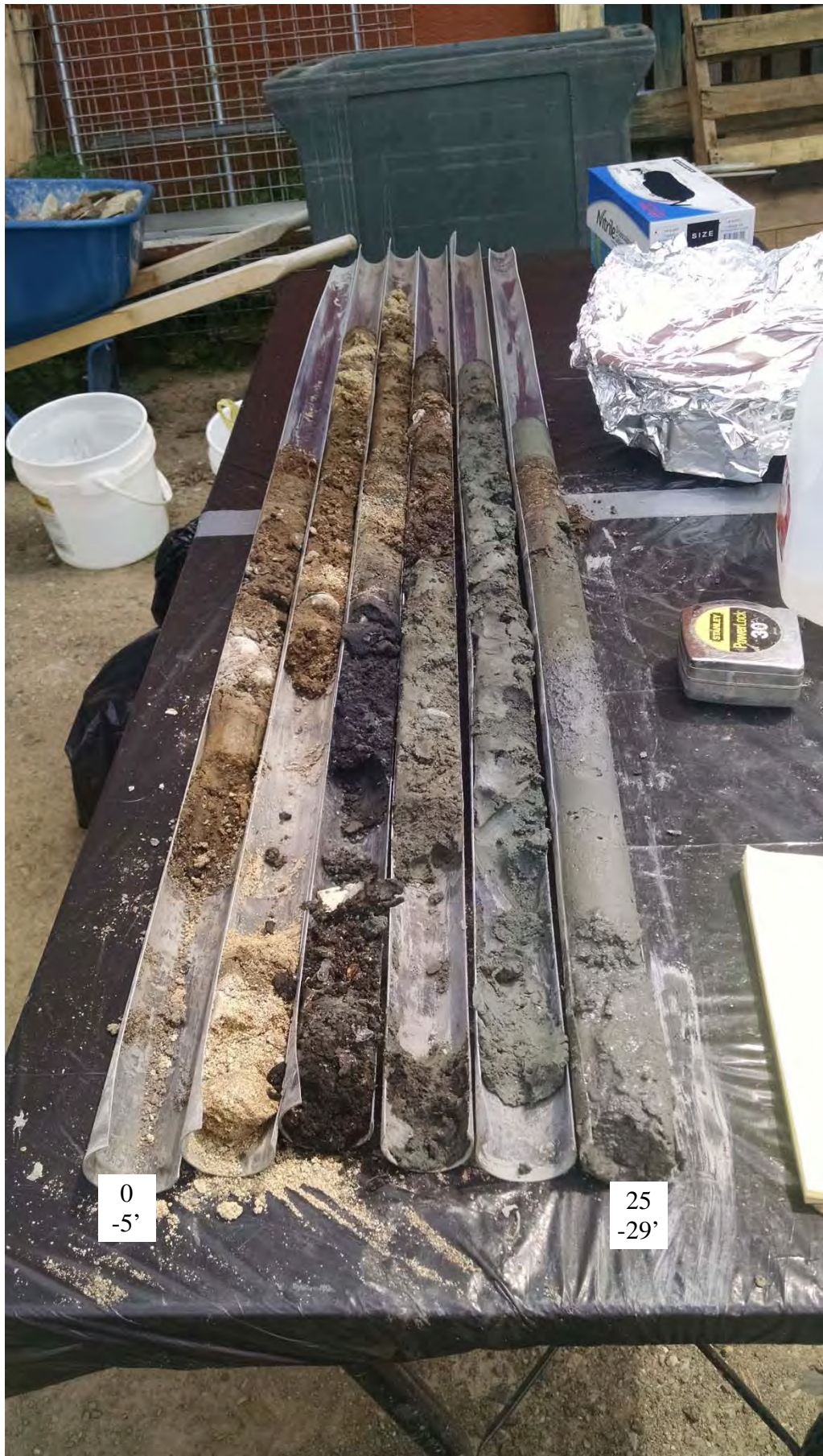
View of soil core from boring SB4. Depth increases from background to foreground, left to right.
