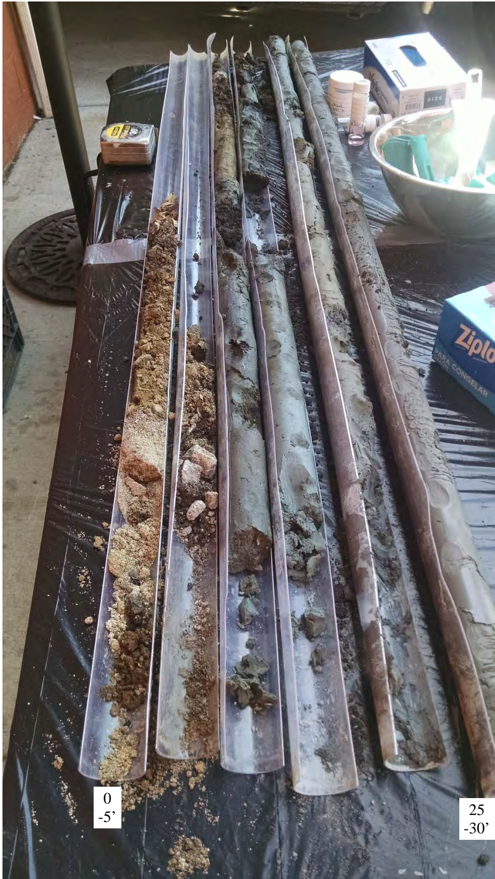
View of soil core from boring SB1. Depth increases from background to foreground, left to right.
