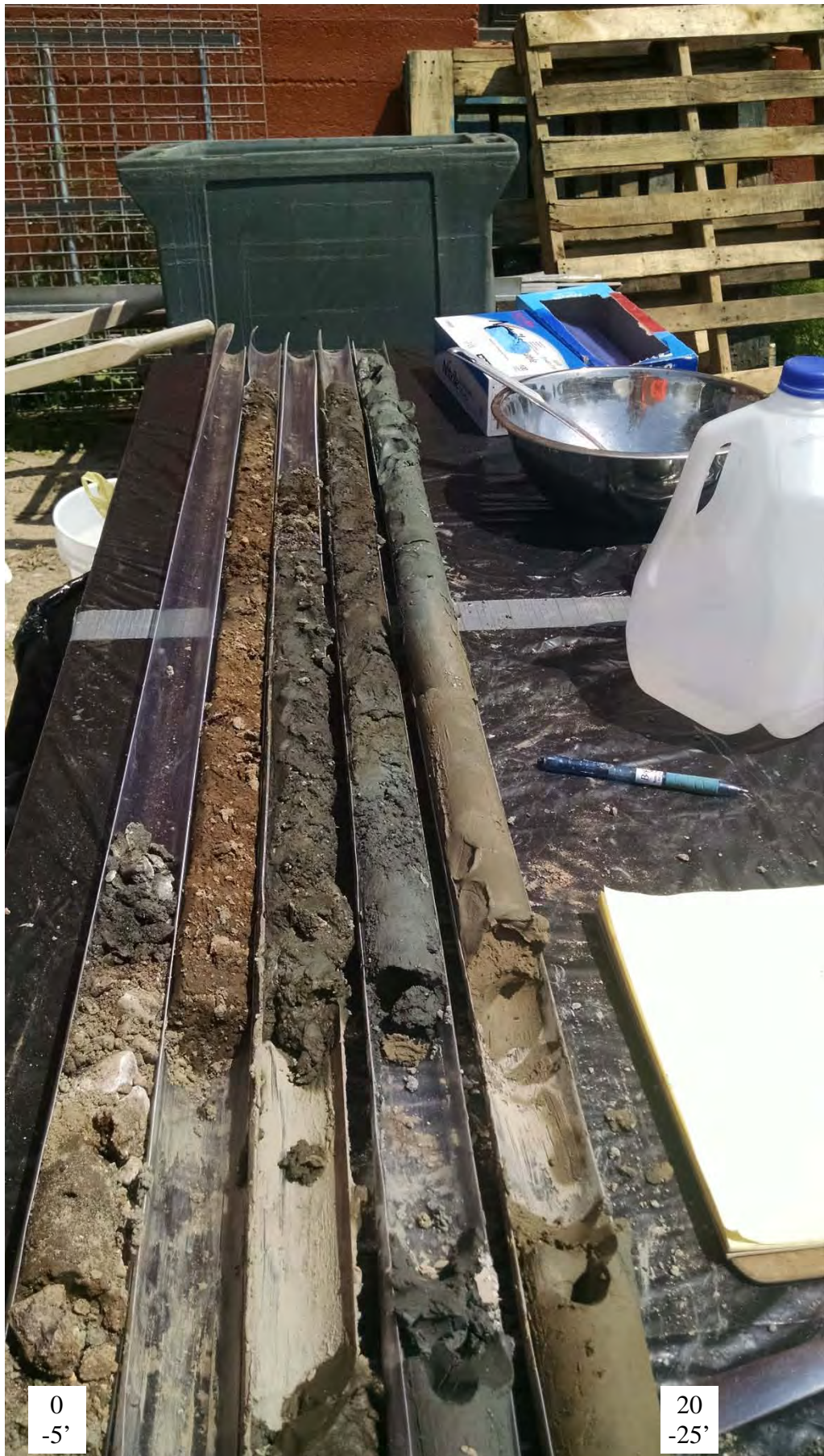
View of soil core from boring SB5. Depth increases from background to foreground, left to right.
