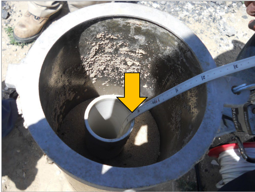
Figure 4: Arrow shows measuring point on a monitoring well, top of casing (©2012, WA Dept. of Ecology).
