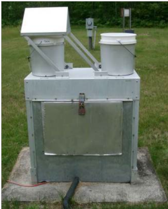
Figure 2: Wet/dry sampler with retractable lid, from the U.S. Department of Agriculture/National Atmospheric Deposition Program (NADP) .
