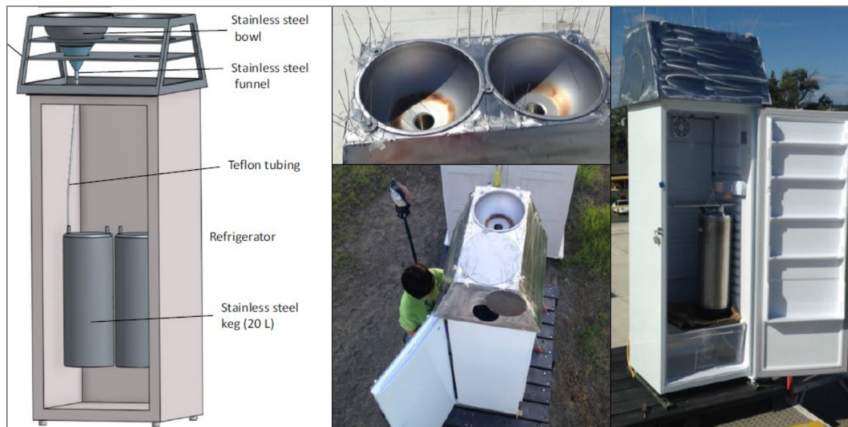
Figure 3: Dual-funnel bulk sampler with refrigerated collector keg, Department of Ecology, Era-Miller, et al., 2019 .
