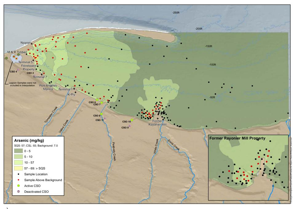
Figure 15. Interpolated Sediment Arsenic Concentrations
