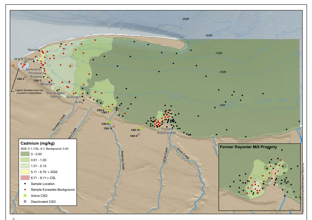
Figure 16. Interpolated Sediment Cadmium Concentrations
