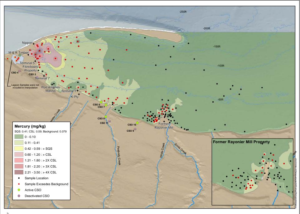
Figure 17. Interpolated Sediment Mercury Concentrations
