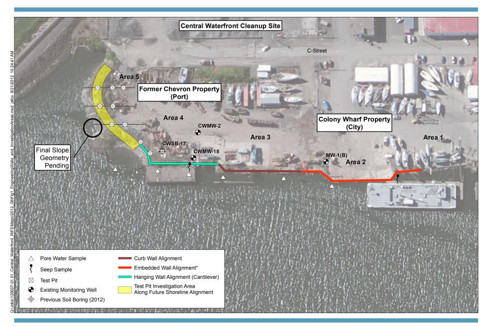
Note \* Embedded wall to be keyed into drift layer and to include tiebacks/soil anchor system.
