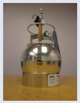
Indoor air monitoring canister (approximately 18 inches tall) used for vapor intrusion testing
