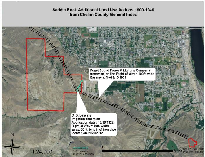
**Figure 11:** 1900-1940 additional land use actions gathered from Chelan County Assessors' Office records drawn on a 1:24,000 scale orthographic projection.
