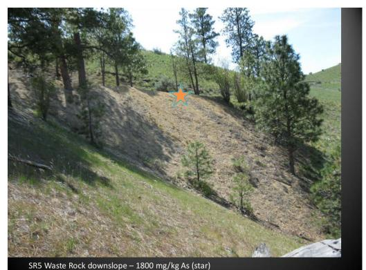
**Figure 31:** Systematic XRF survey of Saddle Rock property; SR5 waste rock pile. Jason Shira, Department of Ecology, 5/4-5/2012.
