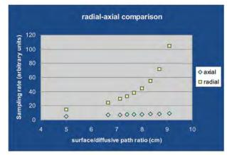
increases linearly with tha ratio of diffusive surface vs diffusive path length, while for the radial simmetry sampler, the corresponding increase is exponential. This means that, let the diffusive surface vs diffusive path length ratio be 8:1, for the axial sampler the uptake rate value is 8 (regardless of dimensions) while for the radial one it is 45.
