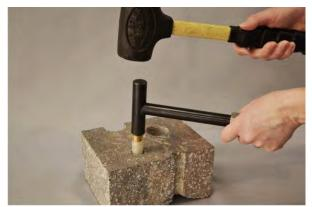
Figure 2. Installing the Vapor Pin<sup>TM</sup>.
