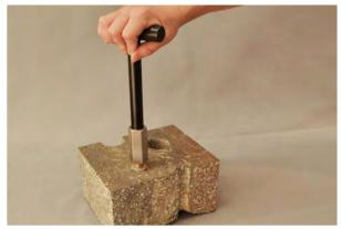
Figure 7. Removing the Vapor Pin<sup>TM</sup>.
