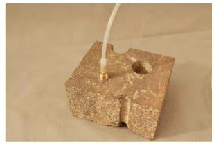
Figure 5. Vapor Pin<sup>TM</sup> sample connection.
