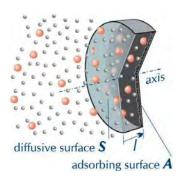
In the diffusive sampler, the adsorbing and the diffusive surfaces are two opposing plane of a closed box. Driven by the concentration gradient, the gaseus molecules (coloured in the figure) pass through the diffusive surface and are trapped from the adsorbing surface.
