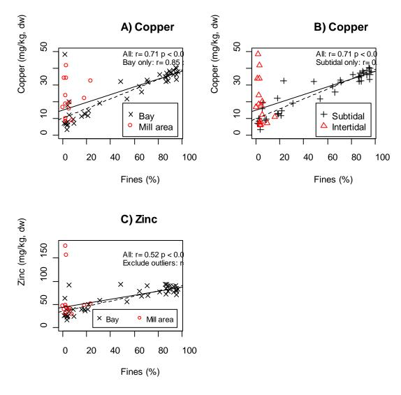
**Figure 5-12.** Correlations between Copper and Zinc Concentrations and the Fine-Grained Sediment Fraction.
