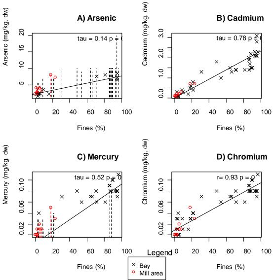
**Figure 5-11.** Correlations between Arsenic, Cadmium, Chromium, and Mercury and the Fine-Grained Sediment Fraction.
