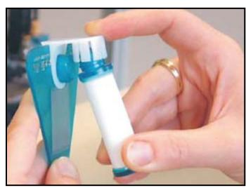
Figure 6: Passive Diffusive Radiello Sampler
