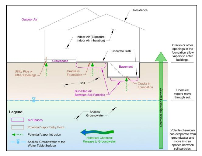
Figure 4: Vapor Intrusion Conceptual Model
