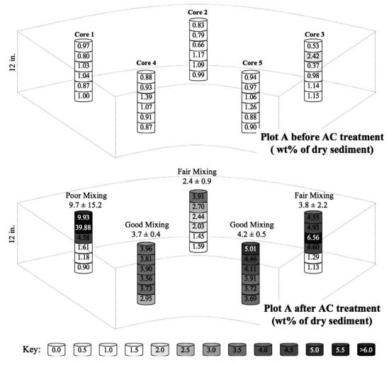
Fig. 4. Comparison of TOC values from sediment cores taken before and after AC treatment in Plot A.
