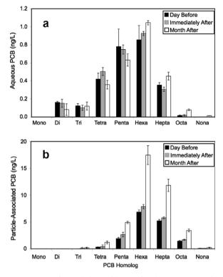
Fig. 8. Comparison of (a) aqueous PCB concentration and (b) particle-associated PCB concentration sampled above Plot A during high tide one day before, immediately after, and one month after AC treatment. Each column and error bar represents the mean and one standard deviation (n = 2).
