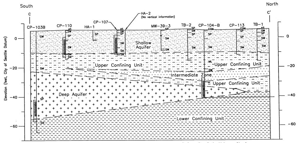
Note: This profile was developed by interpolation between widely spaced borings and monitoring wells. It should be considered as an approximation of geologic conditions to the degree implied by notes on the boring or well logs presented in this report.
