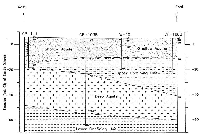
Note: This profile was developed by interpolation between widely spaced borings and monitoring wells. It should be considered as an approximation of geologic conditions to the degree implied by notes on the boring or well logs presented in this report.
