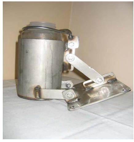
Figure 8. Modified Ecology Sediment Trap
