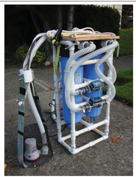
Figure 7. Suspended Solids Filtration Unit
