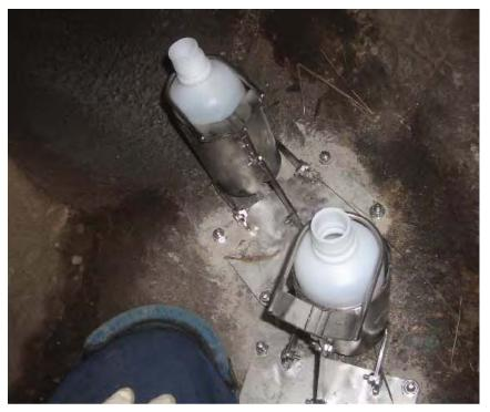
Figure 7. Sediment Traps Installed in a Storm Drain Line
