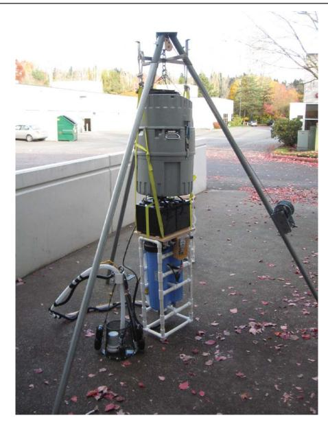
Figure 4. ISCO Whole Water Sampler
