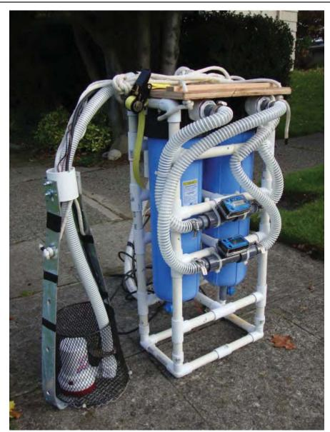
Figure 5. Suspended Solids Filtration Unit
