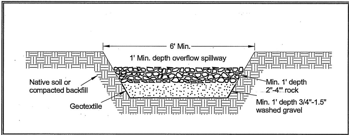
**Figure 4.18 Sediment Trap Outlet**
