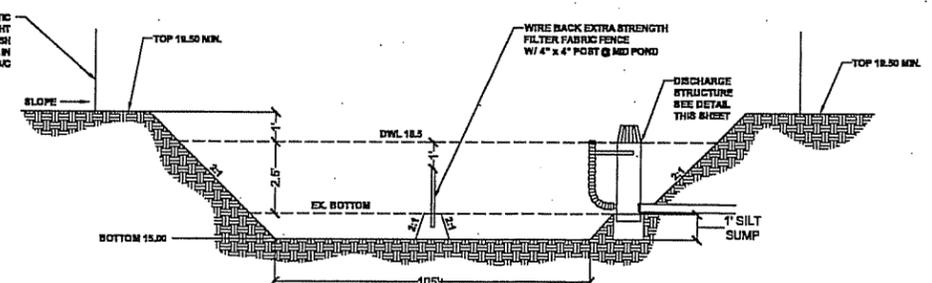
SILTATION / SEDIMENT TRAP #2 SECTION A
