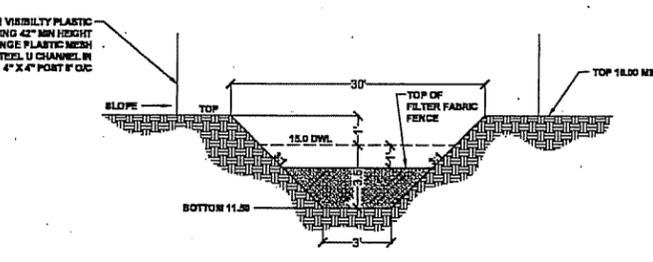
SILTATION / SEDIMENT TRAP #1 SECTION B
