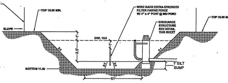
SILTATION / SEDIMENT TRAP #1 SECTION A
