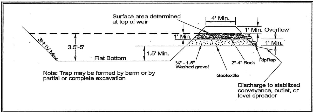
Figure 4.17 Cross Section of Sediment Trap
