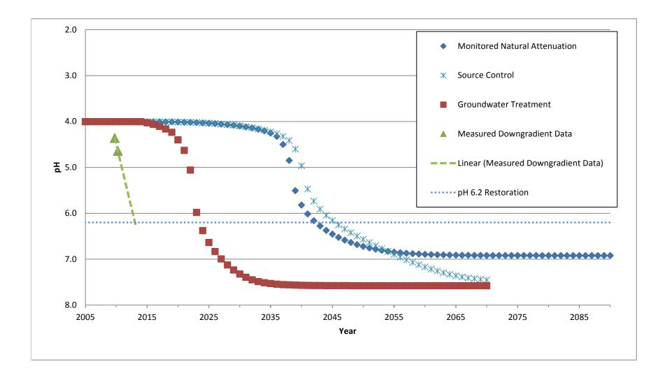
Figure A-2 Modeled Restoration Timeframes under Remediation Alternatives
