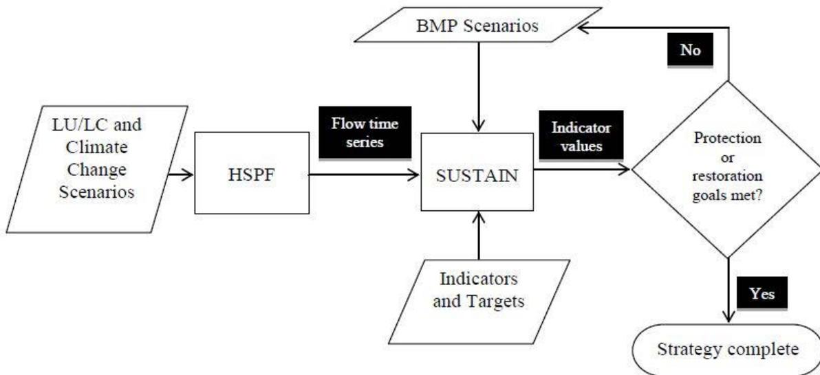
The Hydrologic Simulation Program-FORTRAN (HSPF) model was selected as the watershed model to provide input to SUSTAIN because it has been used by King County as a stormwater management and basin planning tool since the late 1980s. Developing an HSPF model requires inputs that characterize the physical landscape, including land cover, geology, topographic slope,
