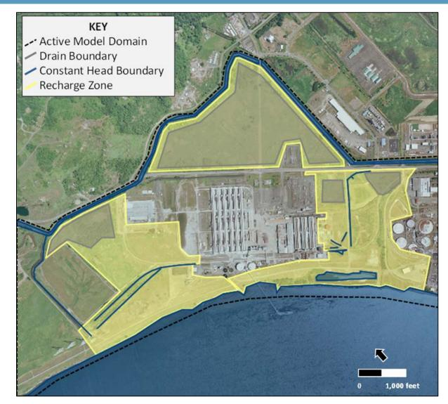
The groundwater flow model domain boundaries include the Columbia River to the south and the CDID ditches to the north and west. Additional model features include the on-site ditches (i.e., U-ditch, cryolite area ditches, and the ditch adjacent to Fill Deposits A, B-1, and B-2 [discharging to 004 Pump Station]) and recharge areas defined within the site. The groundwater flow model also incorporates a drain feature in order to keep water from ponding on the simulated ground surface.
