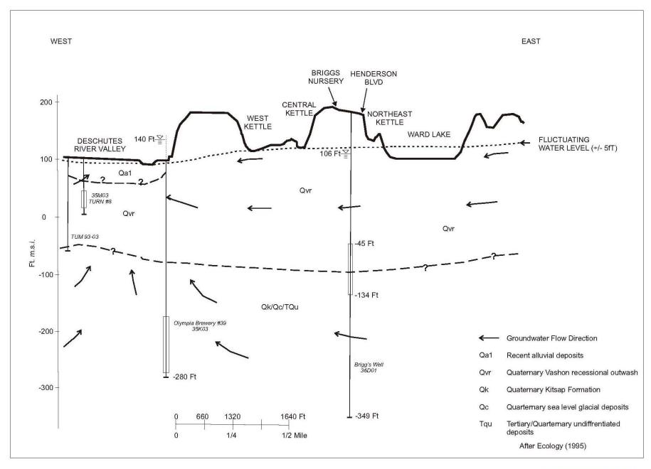
Figure 3. Conceptual Hydrogeologic Cross-Section for Briggs, Tumwater and Surrounding Areas
