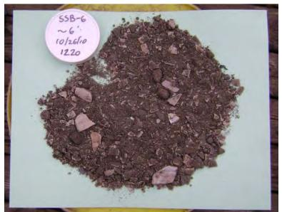
Figure 10. Fragmented shell and sand from SSB-6, about 6 ft. below surface.
