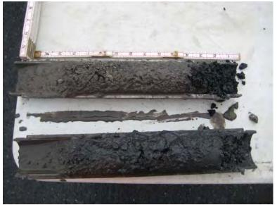
Figure 16. MW-68 core with beach sediments.
