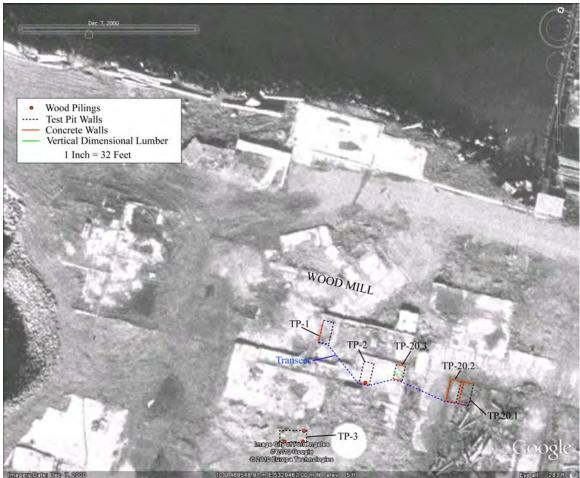
Figure B1. TPs 1, 2, 3, 20.1, 20.2, and 20.3, showing Rayonier mill structural elements.
