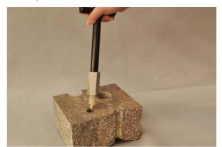
Figure 8. Extracted Vapor Pin<sup>TM</sup>.
