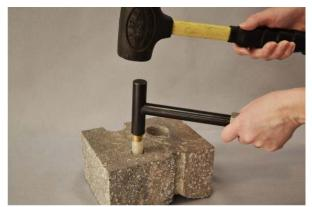
Figure 2. Installing the Vapor Pin<sup>™</sup>.
