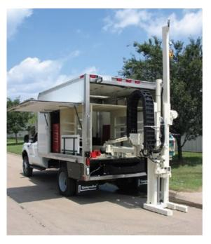
A typical drill rig used for soil air testing.
