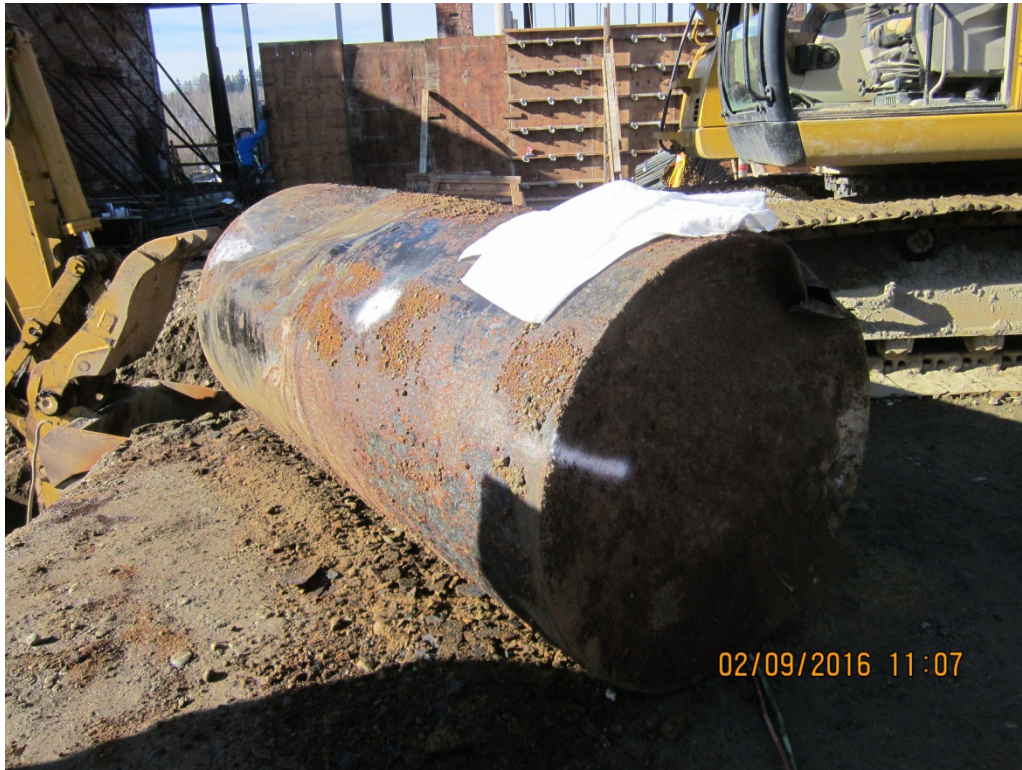
Photograph 7. Looking west at the UST during inspection immediately after its removal.
