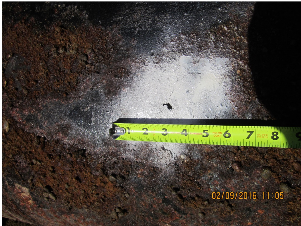
Photograph 5. Close-up view of the 1/2-inch diameter hole observed on the bottom midsection of the UST.
