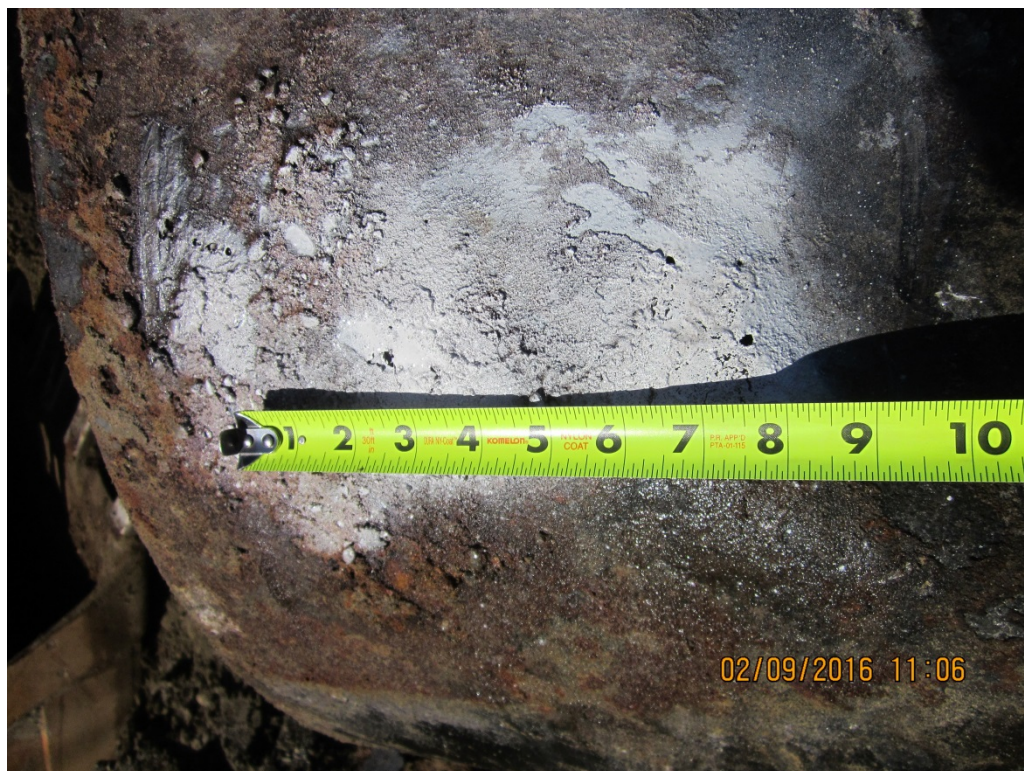
Photograph 6. View of several small holes highlighted with white paint located on the west end of the UST.
