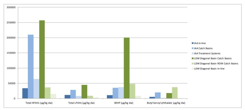
Figure 5. Comparison of maximum HPAH, LPAH, BEHP, and BBP concentrations in stormwater solids
