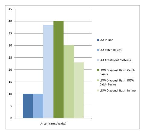
Figure 6. Comparison of maximum arsenic concentrations in stormwater solids
