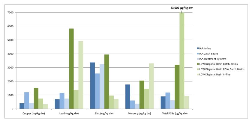
Figure 4. Comparison of maximum copper, lead, zinc, mercury, and PCB concentrations in stormwater solids
