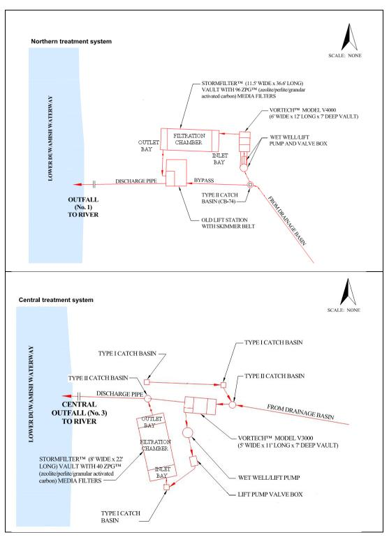
Figure 1. Configuration of northern and central treatment systems
