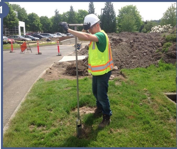
Ecology will enter your yard to collect multiple soil samples using a tool called an auger.
