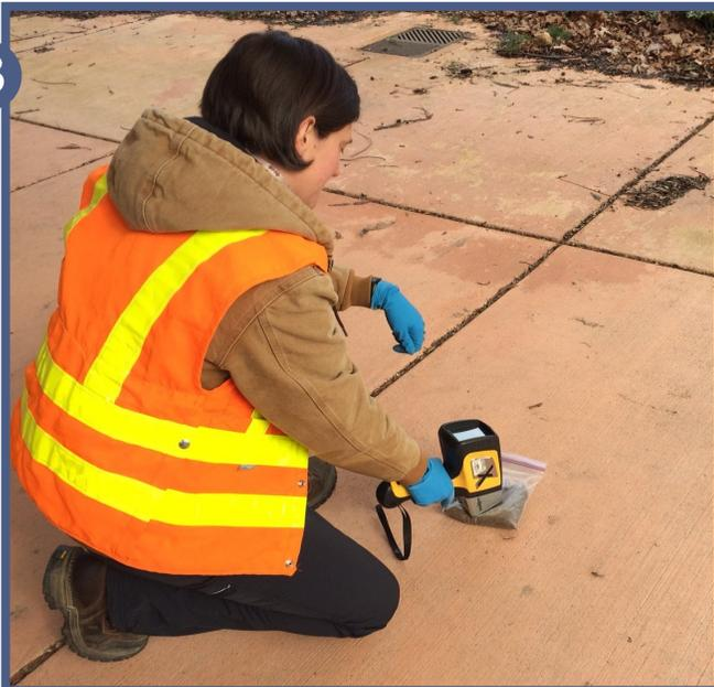
The samples are tested on site using the XRF tool to find out if arsenic is present above state cleanup levels.
