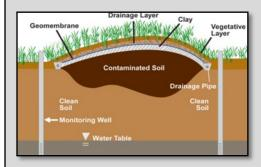
In areas B1, B2, and C4 the plan is to install a cap of a natural or synthetic material over contaminated soil. The cap prevents rain water from entering contaminated soil, and reduces the potential for human exposure. The caps will be new in areas B1, B2, and C4. Already-existing caps will be maintained in areas B3, C5, and C6.
