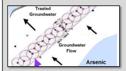
Along the shoreline edge of B2 (not shown on map), the plan is to install a permeable reactive barrier. This barrier is created by injecting chemicals into the ground. The chemicals form a "wall of treatment" that react with arsenic as it passes through the treatment area. Arsenic is then drawn out of groundwater and into soil where it stays in place.
