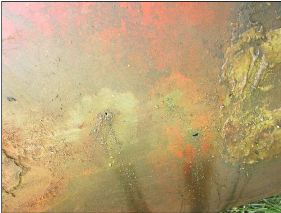
Photograph 5: Close up view of former heating oil AST with small pin holes in bottom of tank.
