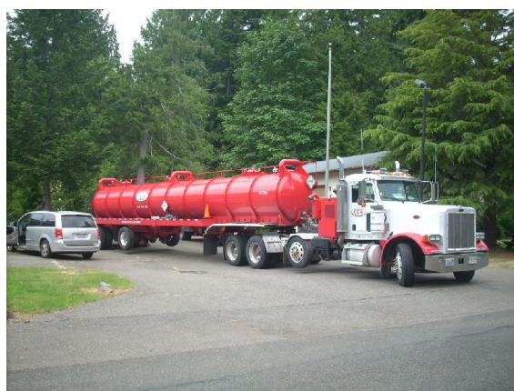
Photo #10: Vac Truck used to remove pit water.
