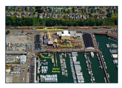
The Marine Railway at the Everett Shipyard, Inc. Site, used to move boats from the water to the shipyard
