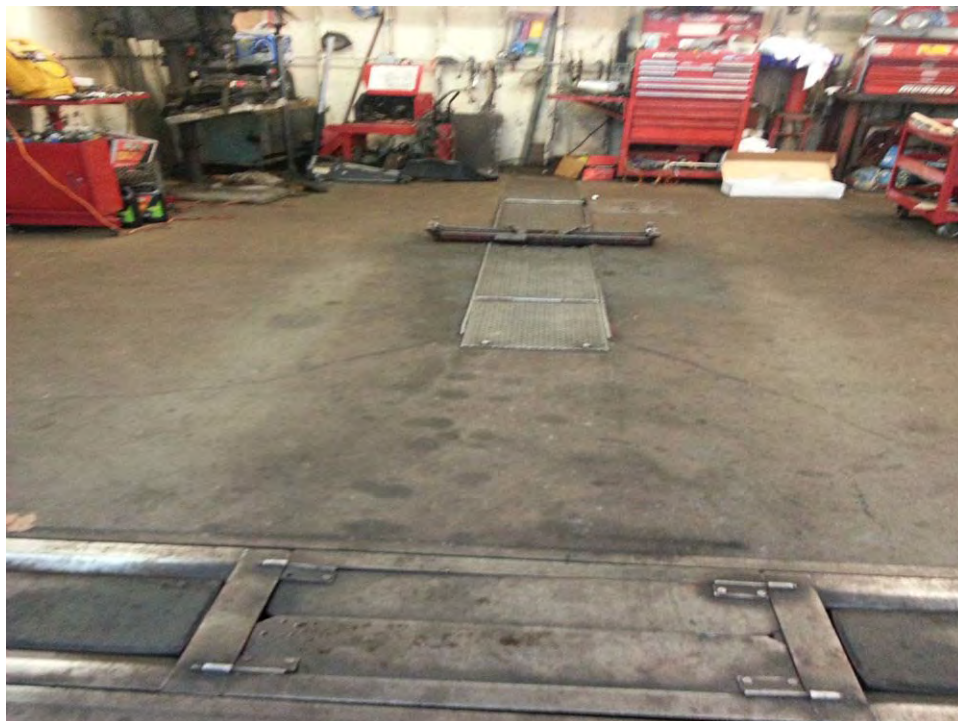
2.) View of one of two hydraulic lift systems in the muffler shop. Each lift had two hydraulic cylinders. (2014 photo)
