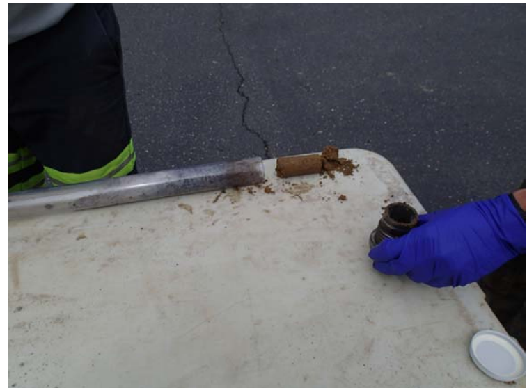
Soil samples were placed into laboratory-prepared sample jars for possible analysis.
