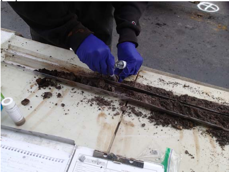
Continuous soil cores retained within plastic sleeves were inspected from the ground surface to total depth at each boring.
