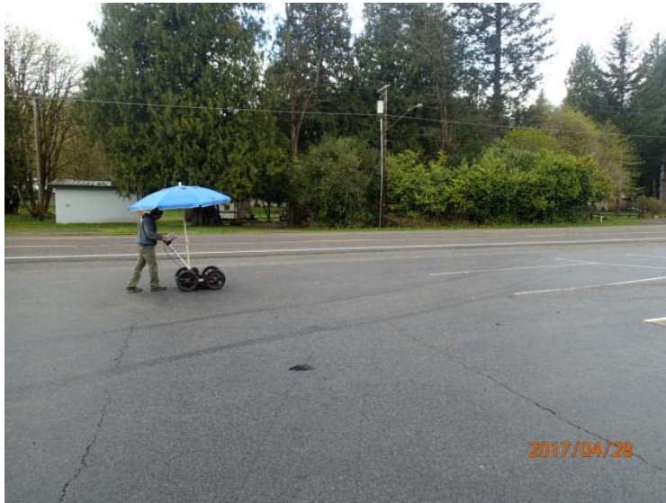
A geophysical survey was conducted to clear boring locations and confirm buried historical features.
