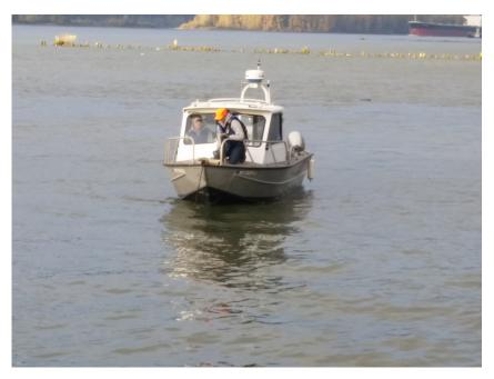
Water quality monitoring vessel deploying instrumentation.
