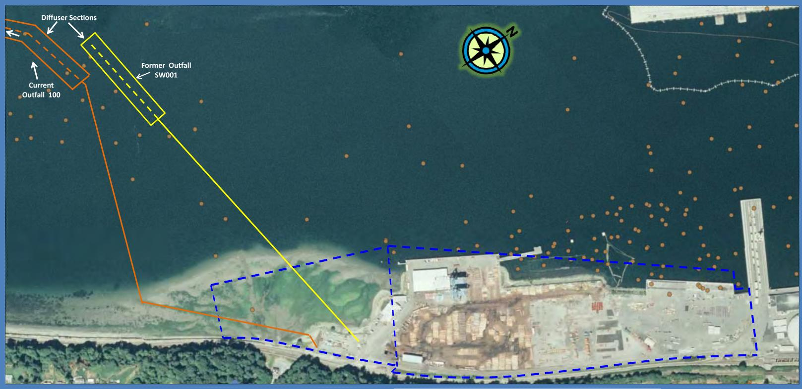
Current Deep Water Outfall 100 Source: Anchor, 2004. Sampling and Analysis Report, Outfall 100 Baseline Sediment Sampling For NPDES Permit #WA00062-01 and Associated Permits. June 2004.
