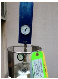
Photograph 6. Flow controller on summa canister used for collecting integrated air samples.
