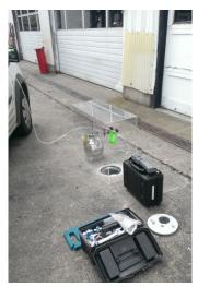
Photograph 3. Setting up soil gas sample Soil Gas 03.
