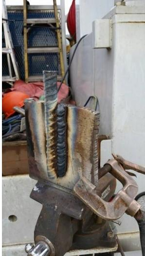
Completed Weld Test Coupon
