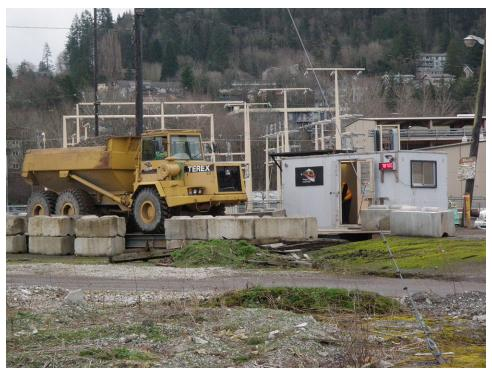
Photograph 19: Temporary weight scale at the Former GP West SSA. Facing south.
