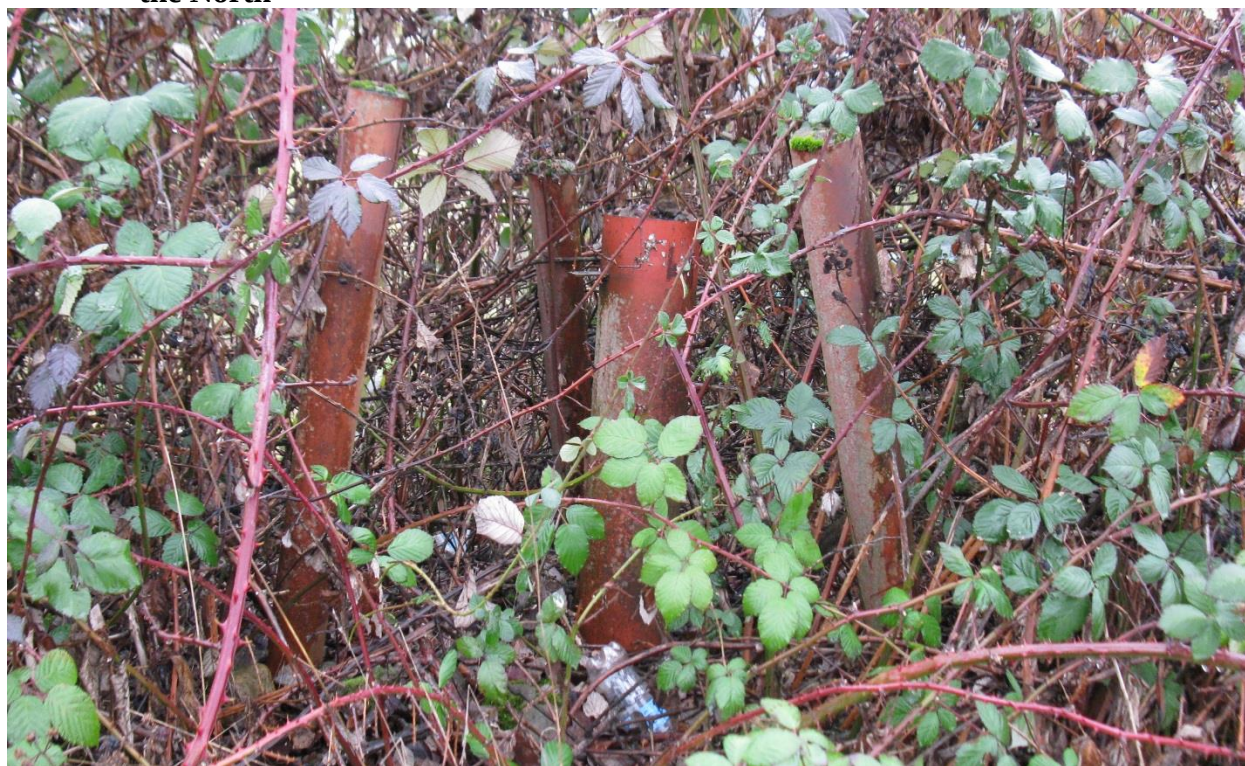
Photo 8: Groundwater Monitoring Well MW-4 that Needs to be Decommissioned - from the North
