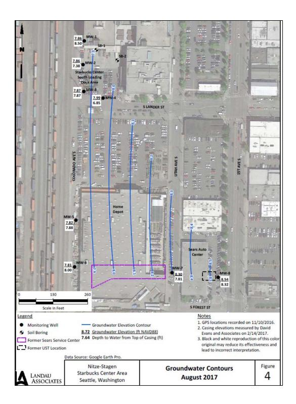
**Figure 3.** Groundwater contour map from 2017 sampling confirming groundwater flow to the west. Monitoring wells used to assess contamination status at multiple cleanup sites close to the Site were included in this sampling event and used to determine groundwater contours. Only data from MW-7 and -8 were used to assess current contaminant conditions at the Site.
