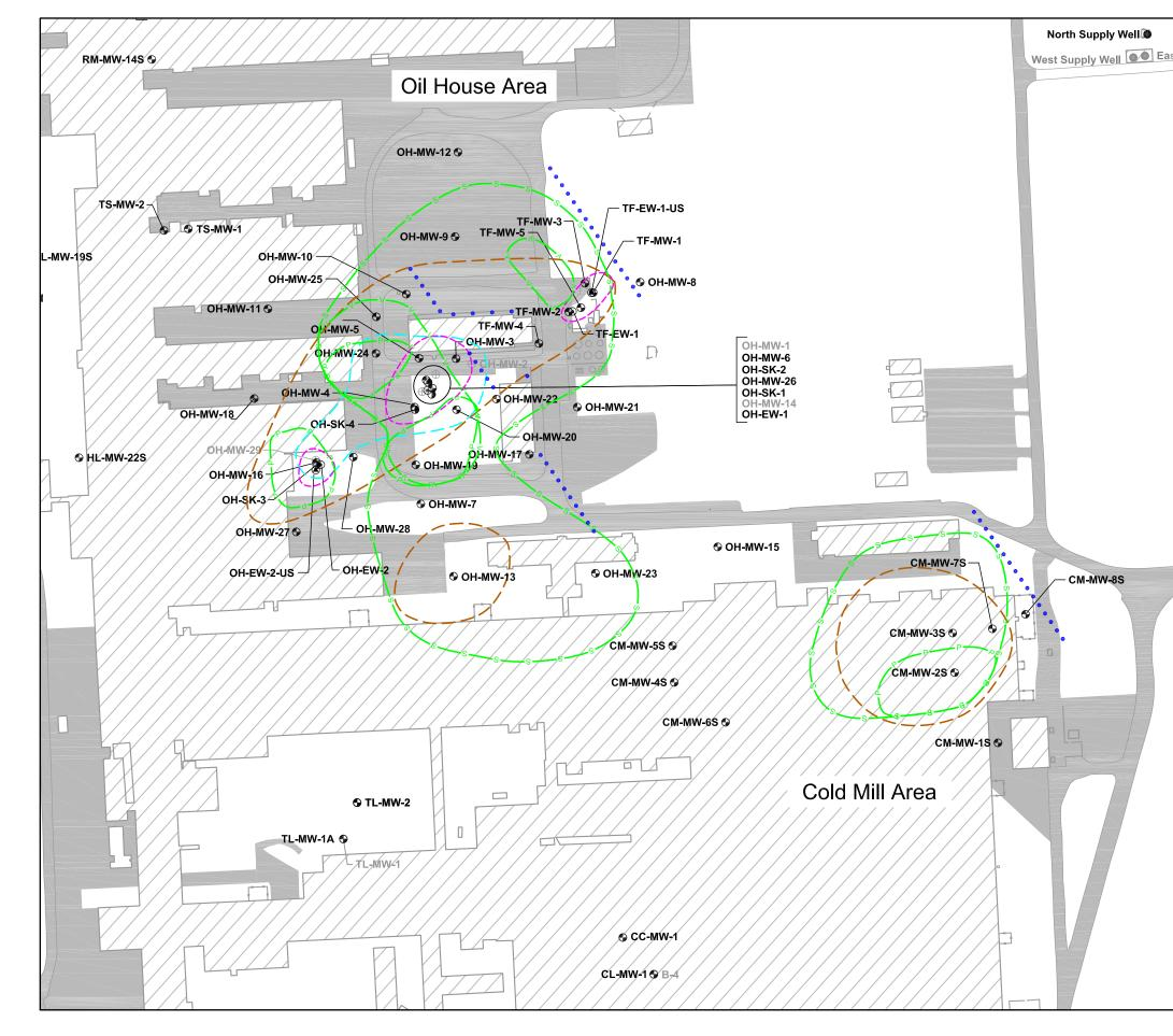
Exploration Location and Number Proposed Injection Well • он-еw-1⊙ Extraction Well он-мw-03 🛛 Monitoring Well TL-MW-3 S Abandoned Monitoring Well он-sк-1 Skimming Well TF-EW-1-US ◎ Upper Screen Well North Supply Well
