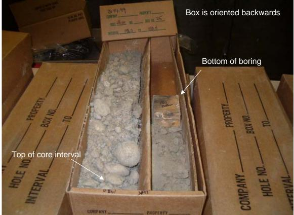
Photograph A-24 - HL-MW-28DD 148 to 150 feet below ground surface.
