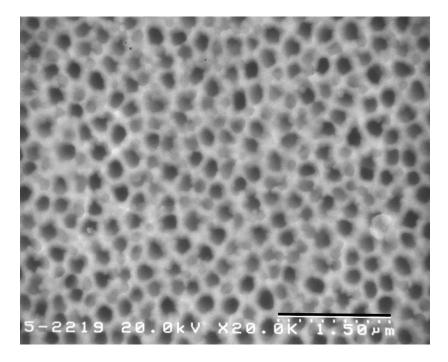
Figure 1. Photomicrograph of aluminum oxide filter surface. Scale bar is 1.5 micrometers in length.
