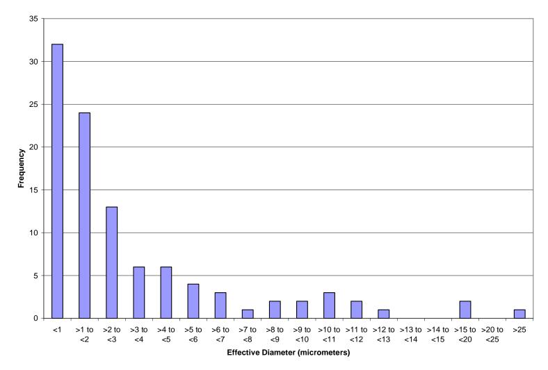
Figure 5. Histogram showing effective diameter from 100 particles in sub-sample A.
