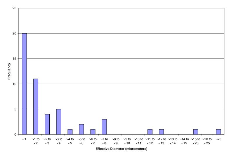
Figure 6. Histogram showing effective diameter of 50 particles in sub-sample B.
