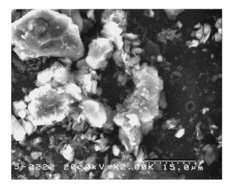
Figure 4. Photomicrograph of aluminum oxide filter surface with particles found on subsample C. Scale bar is 15 micrometers in length.
