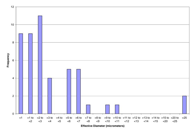
Figure 7. Histogram showing effective diameter of 50 particles in sub-sample C.
