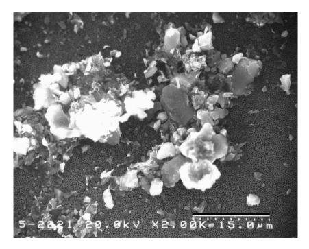
Figure 3. Photomicrograph of aluminum oxide filter surface with particles found on subsample B. Scale bar is 15 micrometers in length.
