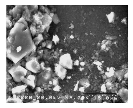
Figure 2. Photomicrograph of aluminum oxide filter surface with particles found on subsample A. Scale bar is 15 micrometers in length.
