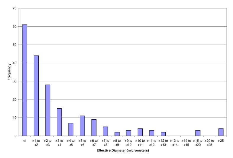
Figure 8. Histogram showing effective diameter of 200 particles in all sub-samples.
