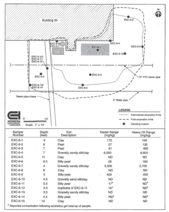
Figure 11. Tank location 6 sampling locations and TPH results.
