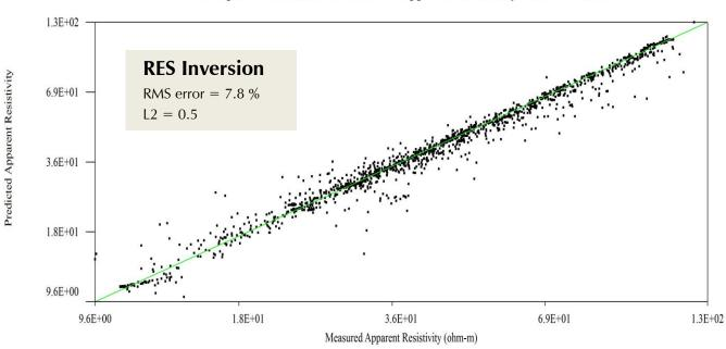
Crossplot of Measured vs Predicted Apparent Resistivity Data for Line 6
