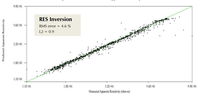
Crossplot of Measured vs Predicted Apparent Resistivity Data for Line 2
