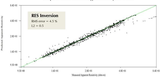
Crossplot of Measured vs Predicted Apparent Resistivity Data for Line 3
