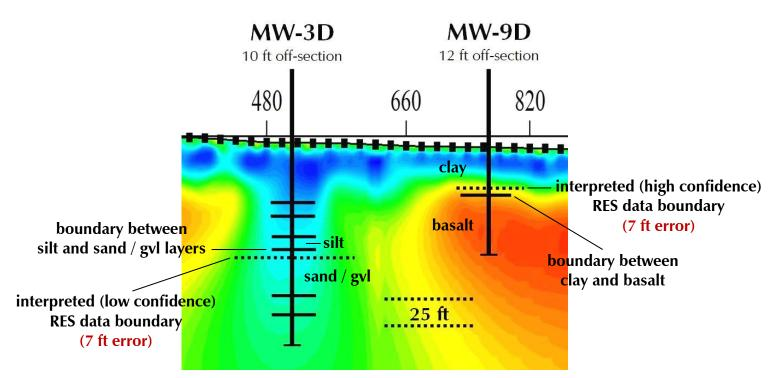
**Figure 1** – Approximate vertical resolution (ie, accuracy) of RES/IP data, as determined from an empirical analysis of the correlation of the data with boring log information.
