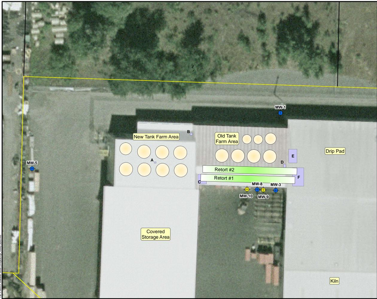
Figure 4 Facility Layout TrueGuard LLC Washougal, Washington
