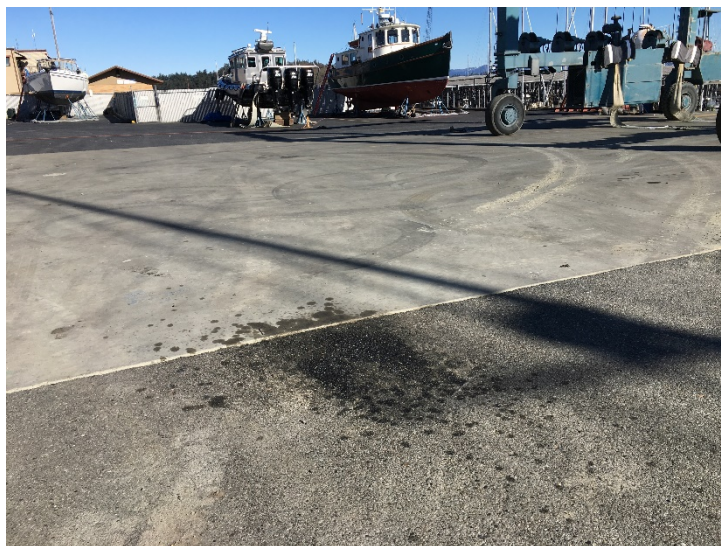
Figure 15 Description: Free liquid present at an oil spill in the yard near the pressure wash pad. A leaking boom truck is likely the source of the spill. Boom truck not present at the facility at the time of the inspection.
