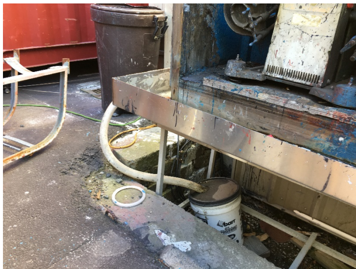
Figure 17 Description: Bucket connected by hose to mixer housing secondary containment. The bucket is full, presumably with commingled stormwater and paint. The trench, which the mixer sits in, is lined with gravel.
