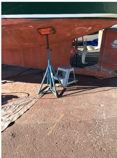
Figure 10 Description: Red dust deposition on ground beneath vessel because the tarp is too short.
