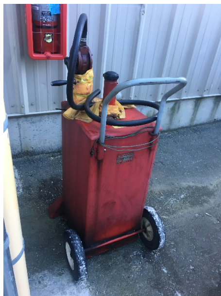
Figure 24 Description: Mobile fueling unit. Absorbent cloth wrapped around the nozzle. Oil residue stains the pavement where the fueling unit sits. Paint residue on the tires.
