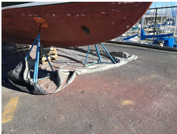
Figure 11 Description: Tarp beneath vessel unsecured and too short to provide adequate cover to collect dust generated from bottom sanding.
